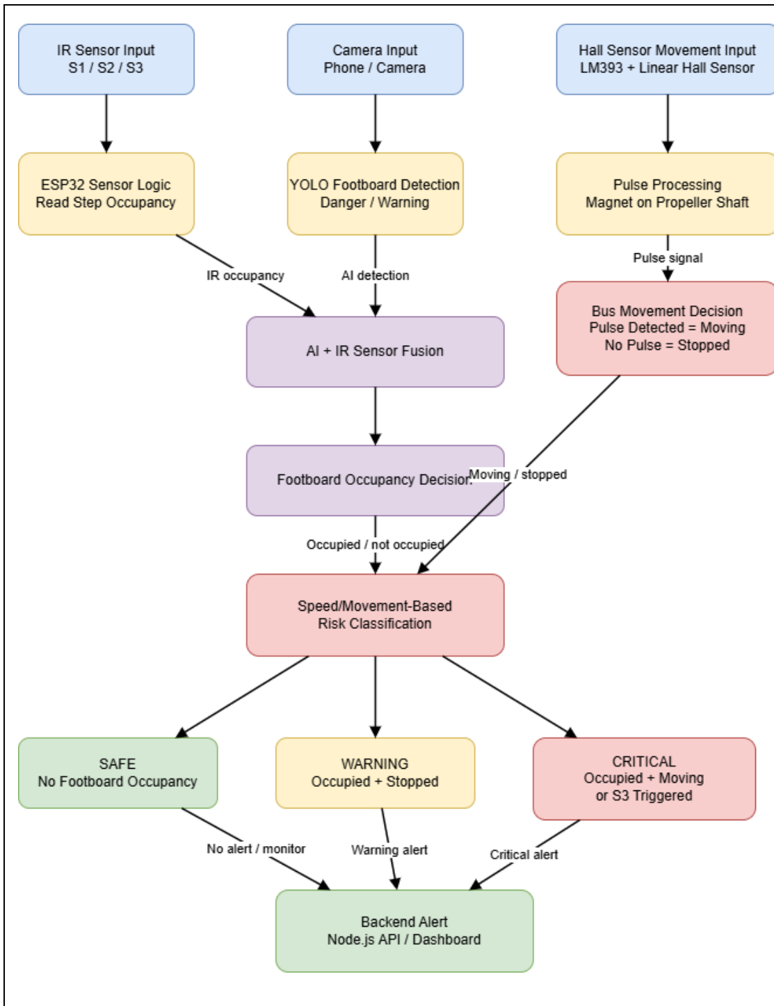
Figure 2.2: Data flow of the footboard safety monitoring module
